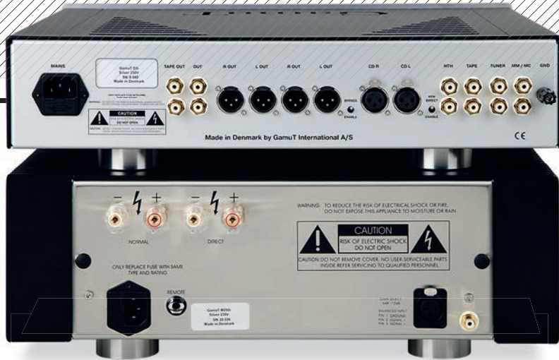
ABOVE: The D3i offers phono and four line inputs (one on balanced XLRs) plus outputs on RCA and dual XLRs. The partnering M250i has RCA and XLR inputs plus Direct and Normal (with a Zobel network) 4mm speaker outputs
