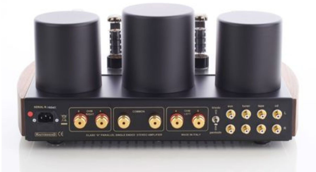
The loudspeaker clamps can be tightened like a vice, for 4 or 8 ohms, a separate secondary winding is available
