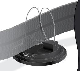
Place flat Loudspeaker Cables between support wings as shown, resting in the crooks of the tension wire supports.
